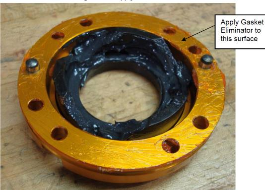
Figure 5.6—Apply Gasket Eliminator
