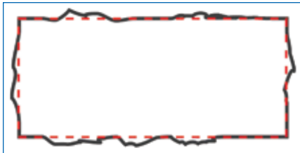
A. Consistent location and part size Inconsistent burr or flash size OK for feed control
