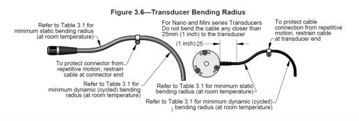
Figure 3.6 from Section 3.3 of Transducer Section Manual
