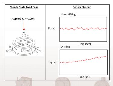
Figure: Example of a simple applied load and data comparison of drifting vs. non-drifting data.
