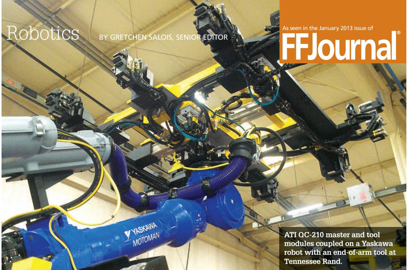
ATI OC-210 master and tool modules coupled on a Yaskawa robot with an end-of-arm tool at Tennessee Rand.
