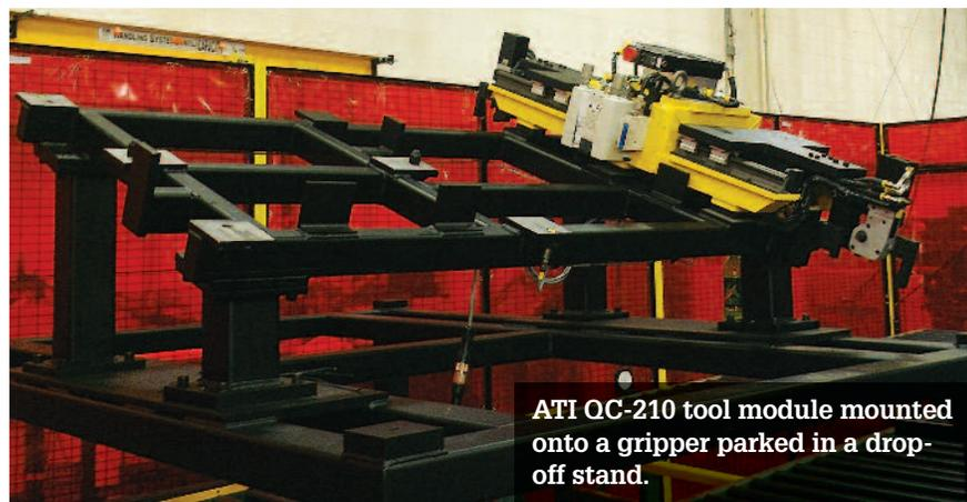
ATI OC-210 tool module mounted onto a gripper parked in a drop-off stand.
