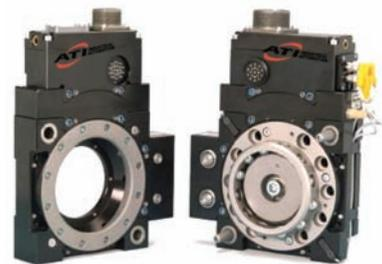
An end effector with two mating parts, a master side (left) and tool side (right), is designed to automatically lock together and pass utilities such as electrical signals, pneumatics, and water.
