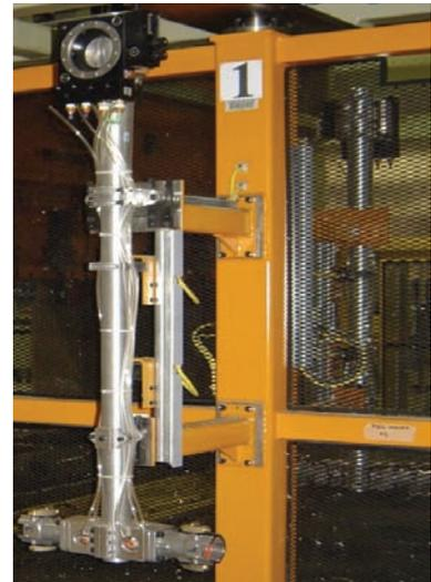
The master side of the tool changer mounts to a robot or other structure, offering tool change flexibility.
