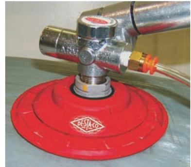
Vacuum cups are available to handle parts with a variety of surface conditions and flat, mild, or high contours.
