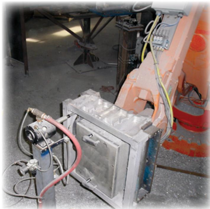
**When the aluminum casting comes out of the V-process, there are minor flashings that need to be removed. Harmony Castings LLC/TPi ARCADE uses ATI’s Flexdebur model RC-660 mounted in a stationary position and a robot to maneuver the part for deburring.**
