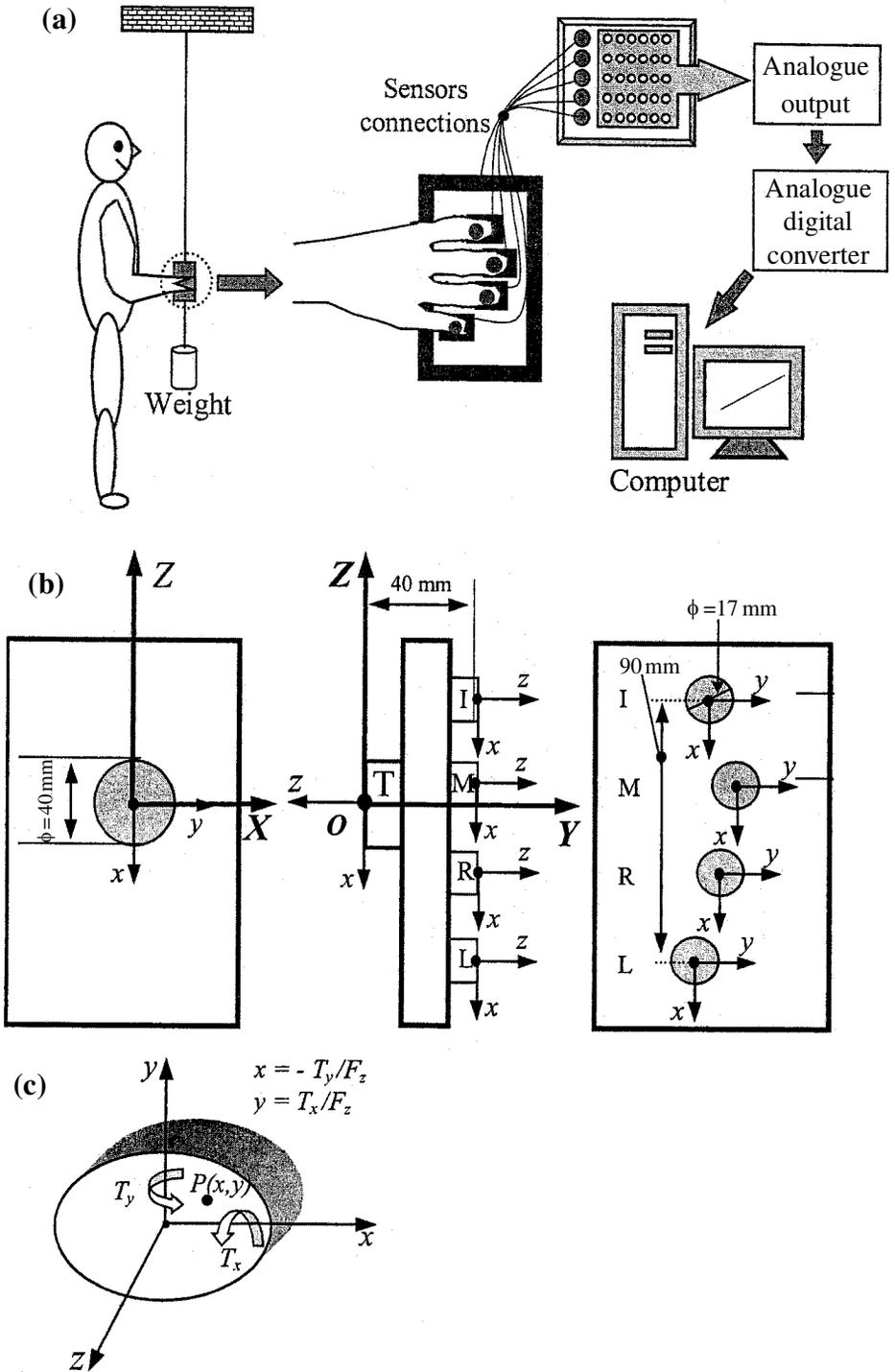
Figure 1. A schematic illustration of the experimental set-up: (a) Task performance and data collection; (b) Instrumented handle with 5 force sensors viewed from the thumb side, the edge side, and the finger side. Each sensor has its own local co-ordinate system that originates from the centre of the gripping surface; (c) Force and torque designation on
