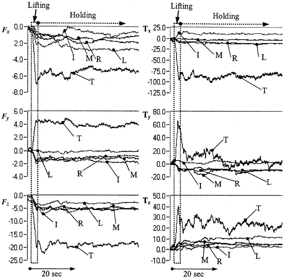
Figure 2. Force and torque traces while lifting and holding the heavy load (10.4 N) weight. Unit for force is N. Unit for torque is N-mm. Note that only a portion (20 s) of the holding phase is shown. The data are represented in their local co-ordinates.
