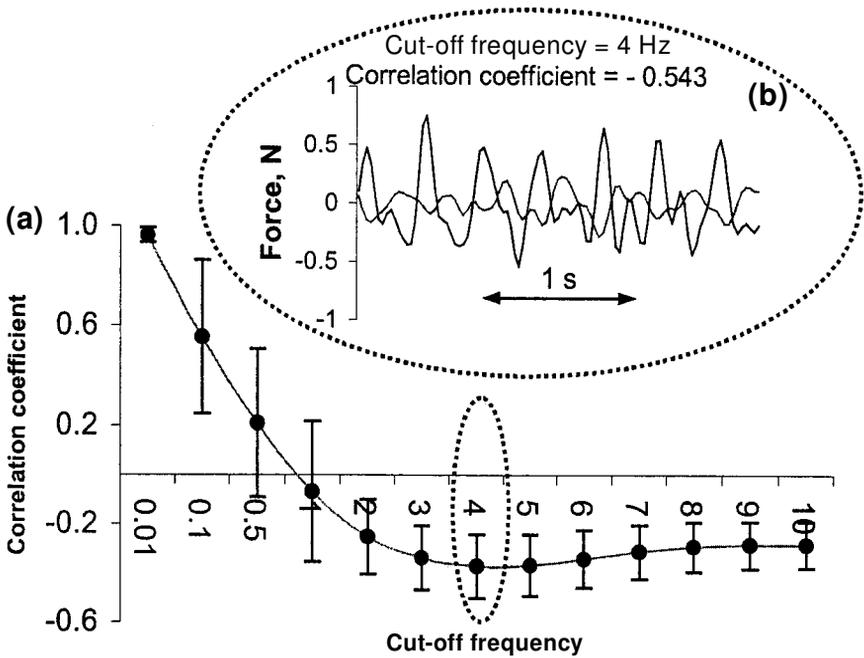
Figure 4. (a) Correlation of the normal force of the thumb and the sum of the normal forces of the four fingers after filtering using high-pass filter at different frequencies (a period of 50 s). Mean of median value  $\pm$  SE from 8 participants. (b) A zoom-in graph (1 s) showing the anti-phase relationship (negative correlation) between the two force traces for a representative subject.
