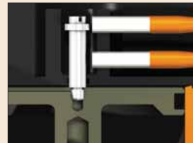
Figure 4: Close-up of SIP in Unlock position. Unlock sensor activated by the detection shaft. Lock sensor is not activated.
