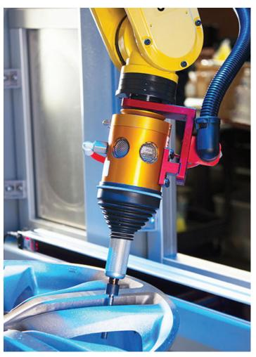
ATI's deburring tool in action with iA-Robotics
