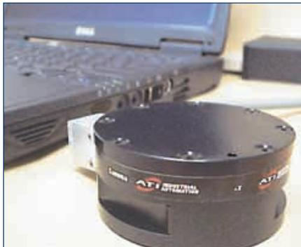
**DAQ F/T sensors are currently compatible with PCI, cPCI, PCMCIA, ISA, and USB data-acquisition cards with a variety of resolutions and sampling rates.**
