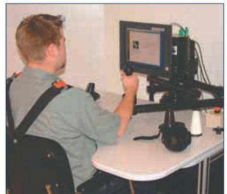
**MIT's Newman Laboratory for Biomechanics uses a rehabilitation robot equipped with an F/T sensor to significantly improve patients' recovery of arm movement following strokes.**
