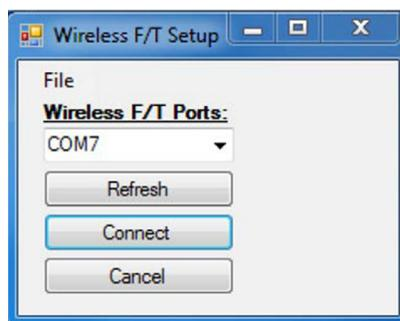
7. Select the COM port corresponding to your Wireless F/T and press the connect button. You may need to press the “Refresh” button if no COM ports are shown.
