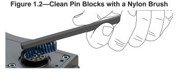
6. Inspect the Master and Tool pin blocks for stuck pins or pin block damage.
