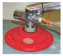
Vacuum cups are available to handle parts with a variety of surface conditions and flat, mild, or high contours.
