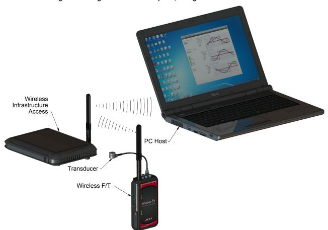
Figure 2.1—Signal Path to a Computer, Using a Wireless Access Point
