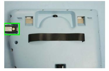
Figure 4.1—Insert USB Drive into USB Port on the Teach Pendant
