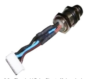
Figure 5-5— Threshold Relay Pico-to-Molex wire harness
