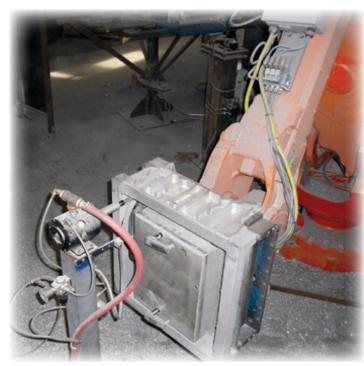
When the aluminum casting comes out of the Vprocess, there are minor flashings that need to be removed. Harmony Castings LLC/TPi ARCADE uses ATI's Flexdeburr model RC-660 mounted in a stationary position and a robot to maneuver the part for deburring.
