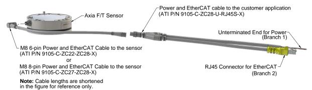
Figure 3.2—Axia130 Cable Configuration
