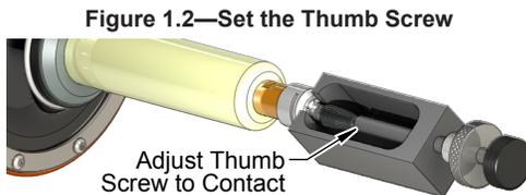
4. Tighten the jam nut against the fixture to secure the thumb screw position. Then remove the fixture.
