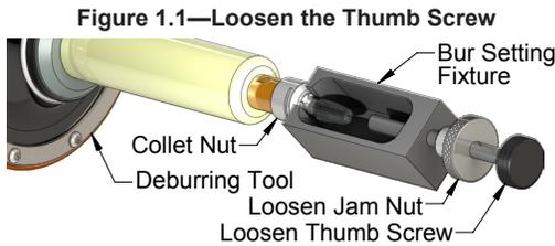
3. While holding the fixture against the collet nut, adjust the thumb screw until it contacts the tip of the cutting bur.
