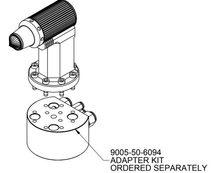
2. CUSTOMER TO SUPPLY M6 FASTENERS AND DOWEL FOR ADAPTER PLATE MOUNTING.
