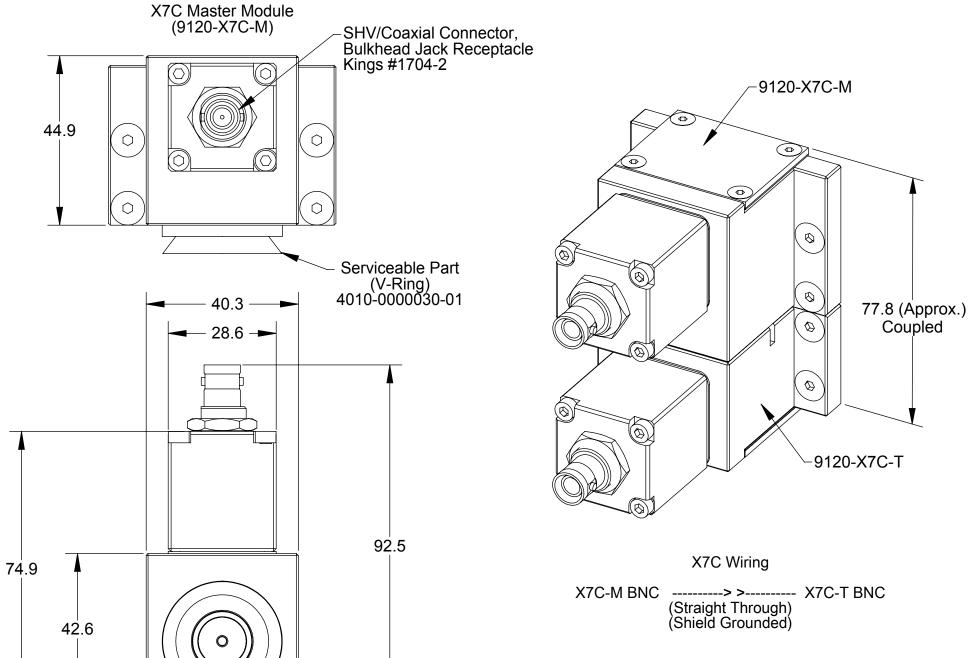
Internal Wiring = COAX Cable (apx. 0.7 ft)
