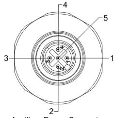
Auxiliary Power Connector Turck #FK 4.5-0.2/14.5/NPT (Tool Side) Scale 2:1
