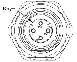
Profinet Connector 120404-04-064 (Master and Tool Side) Scale 2.5:1
