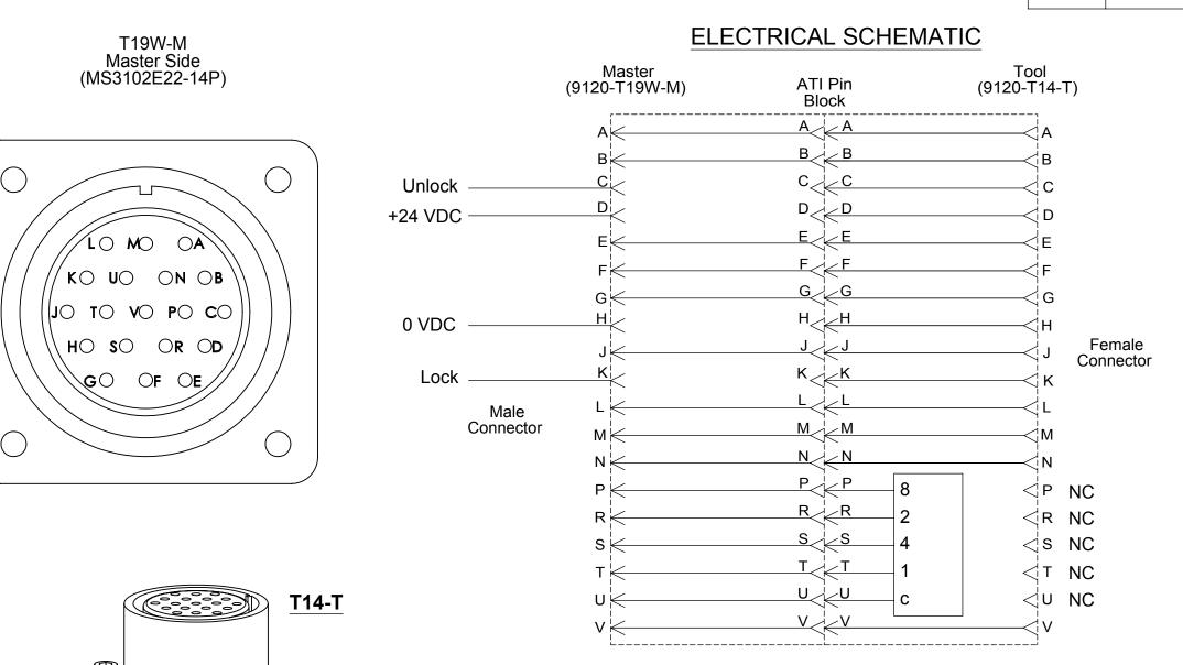
Signal Legend Pin V: 0 VDC (recommended) Pin U: 5-50 VDC 100mA Max (Tool ID)
