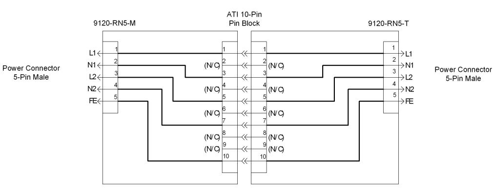
1. ATI Pin Block pin #10 is "First to Mate and "Last to Break" contact. recommended as ground.
