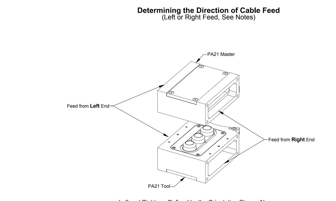
Left and Right are Defined by the Orientation Shown Above with the Master Module on Top and the Tool Module Below.
