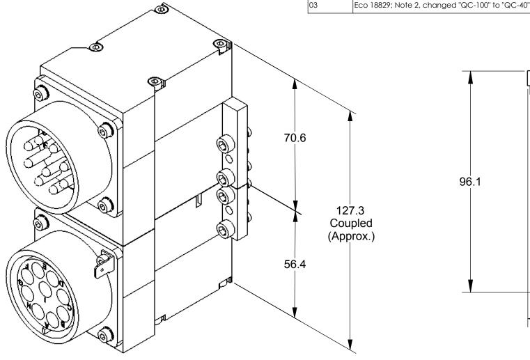
MT9 Pin Out MT9A Master MT9A Tool SG3102E28-84P SG3102E28-84S Male Connector Female Connector A ----- >> ----- A B ----- >> ----- B C----- >> ----- C H------ >> ------ H |------|
