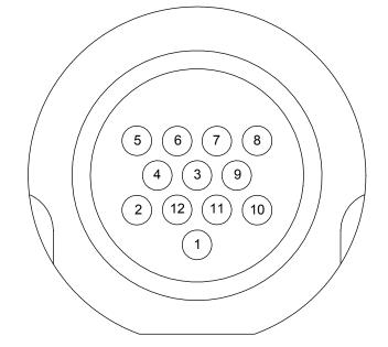
12-Pin Pin Block DETAIL B SCALE 3:1
