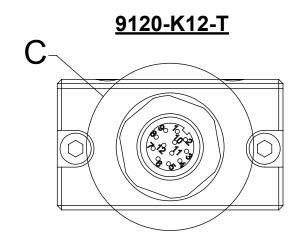
12-Pin Male Connector DETAIL A SCALE 3: 1
