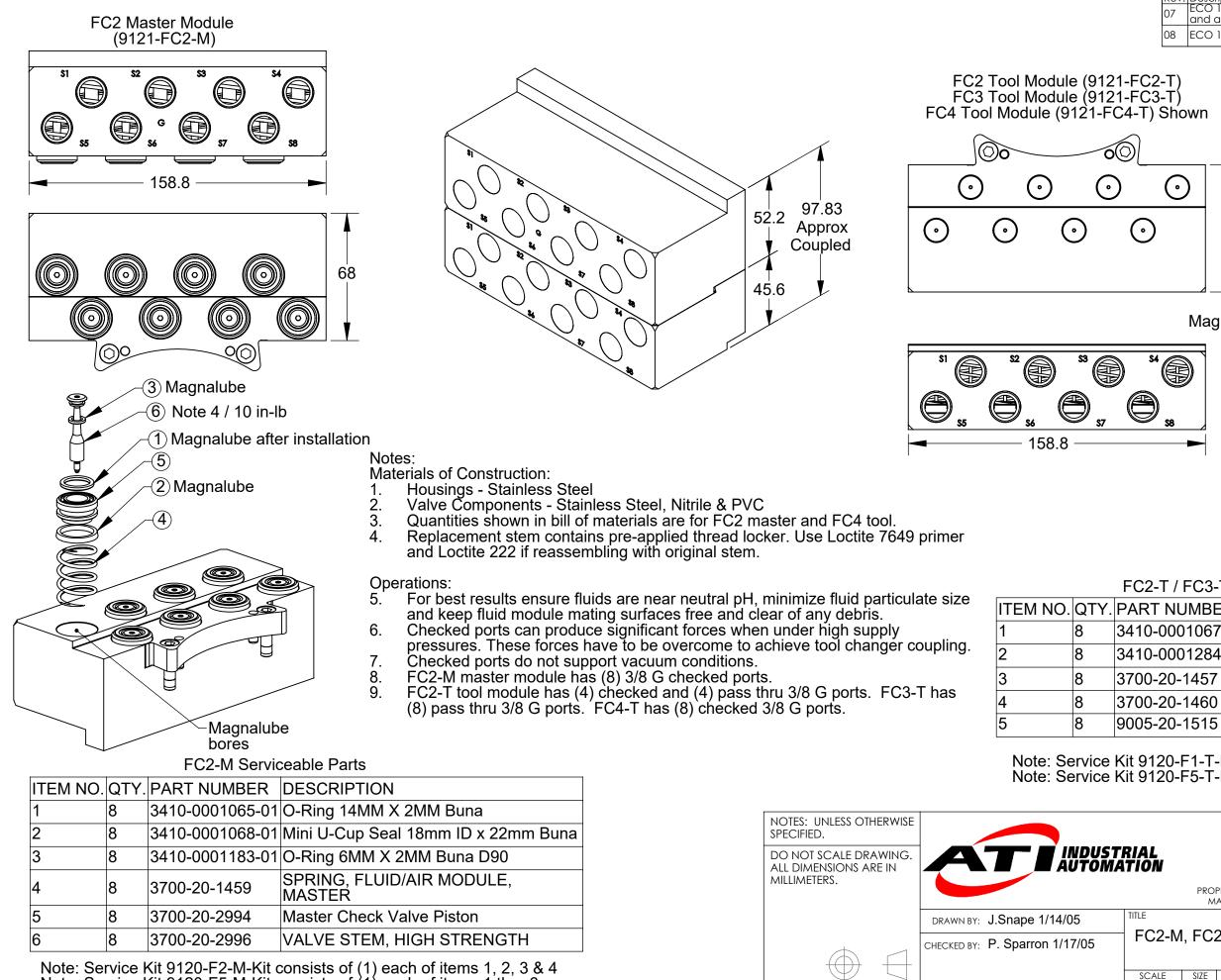
Note: Service Kit 9120-F2-M-Kit consists of (1) each of items 1, 2, 3 & 4 Note: Service Kit 9120-F5-M-Kit consists of (1) each of items 1 thru 6
