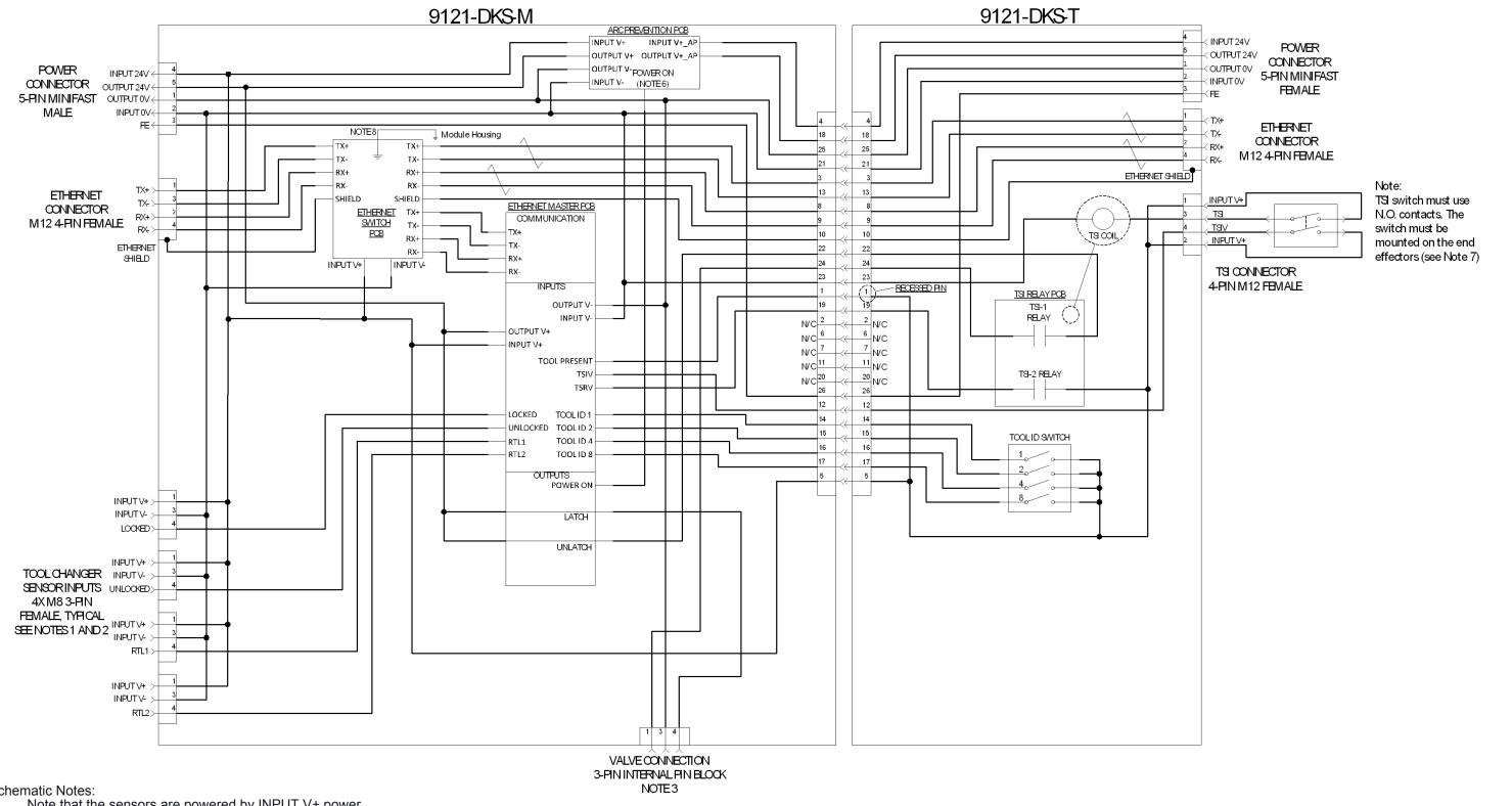
Note that the sensors are powered by INPUT V+ power.
