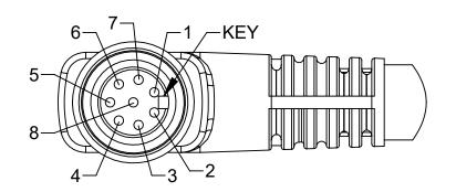
VIEW B-B MASTER 8-PIN FEMALE M8 CONNECTOR BINDER #77-3408-0000-50008 SCALE 3:1
