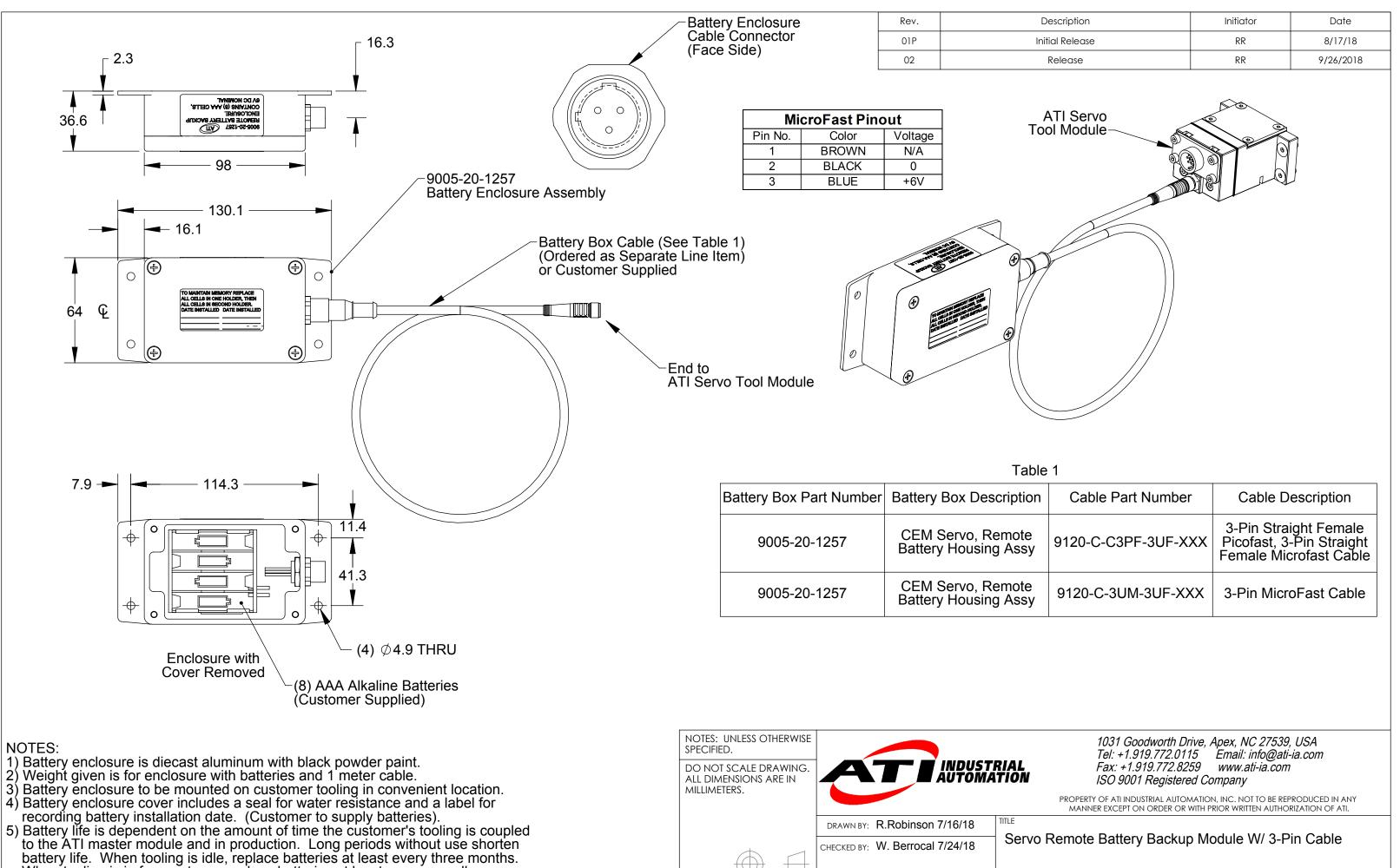
When tooling is in frequent use, replace batteries at least once annually.
