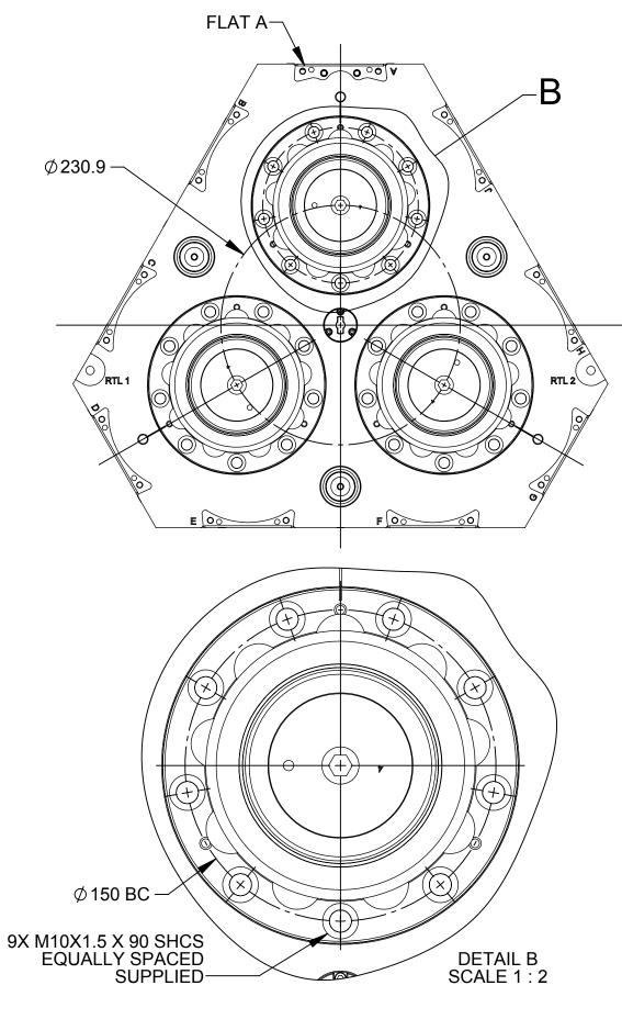
M10 SHCS MOUNTING PATTERN, 3X EQUALLY SPACED
