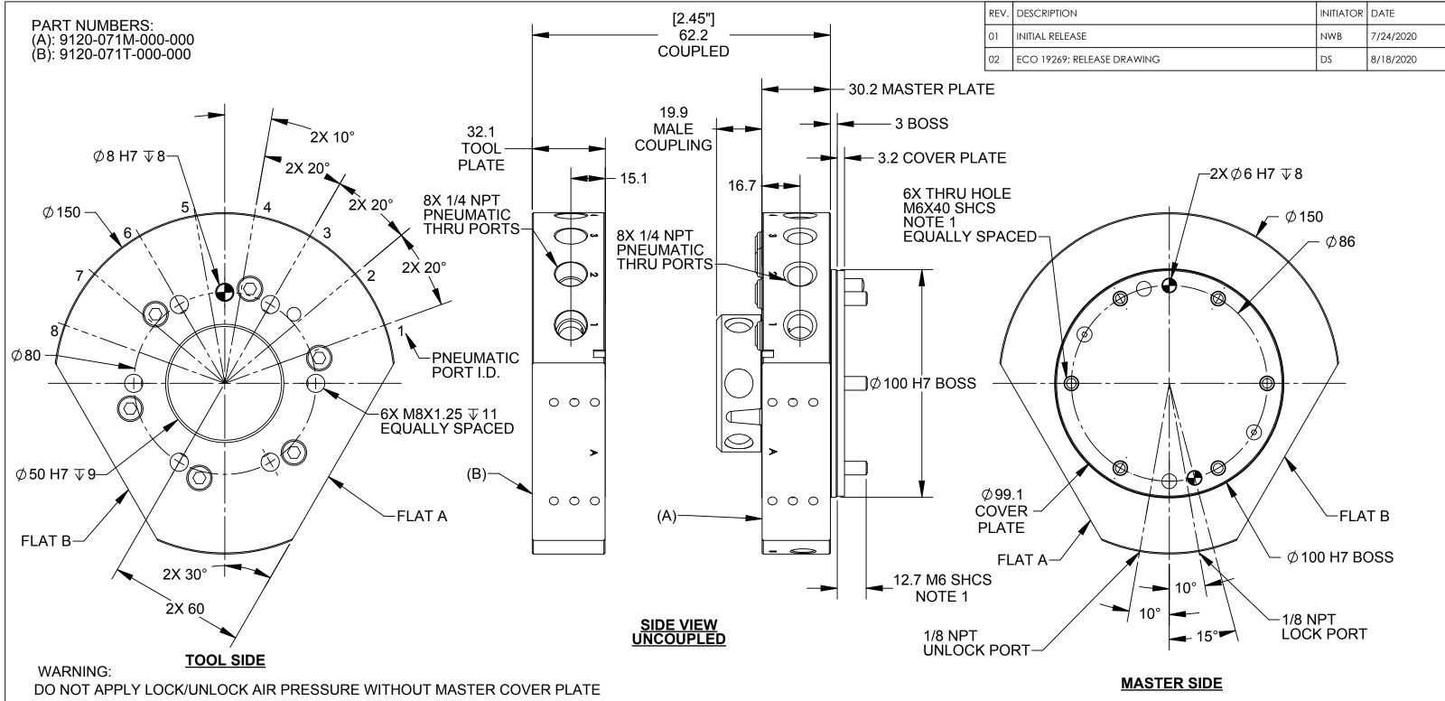
PROPERLY ATTACHED. IF COVER PLATE IS NOT USED, MASTER SHOULD BE PROPERLY ATTACHED TO INTERFACE. FAILURE TO DO SO COULD RESULT IN DAMAGE TO COVER PLATE AND O-RING.
