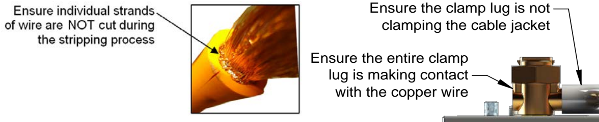
Figure 2.3—Wire Stripping and Clamping
