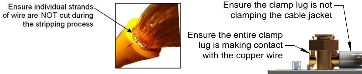
Figure 2.3—Wire Stripping and Clamping
