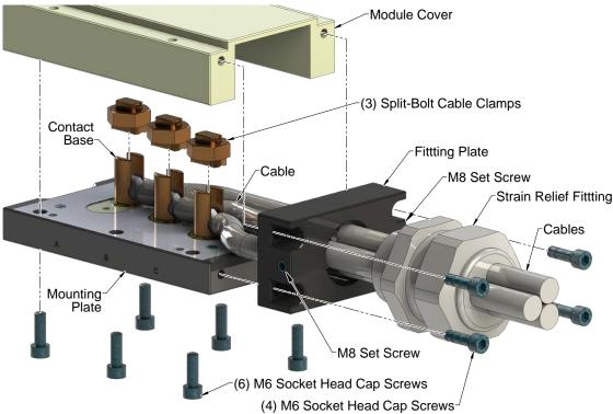
Figure 2.4—Module, Fitting Plate, and Strain Relief
