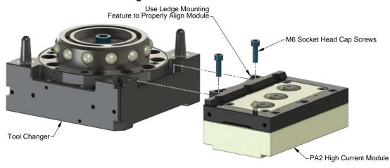
Figure 2.5—Module Installation
