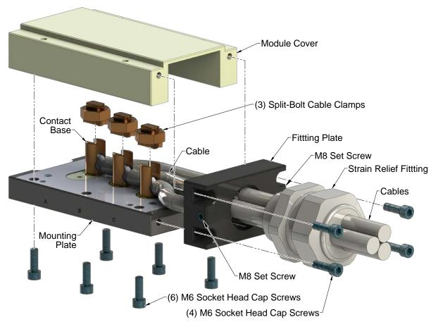
Figure 2.1—Module, Fitting Plate, and Strain Relief
