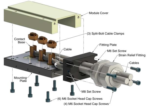
Figure 2.1—Module, Fitting Plate, and Strain Relief
