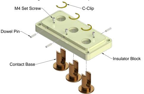
Figure 5.4—Contact Base Replacement
