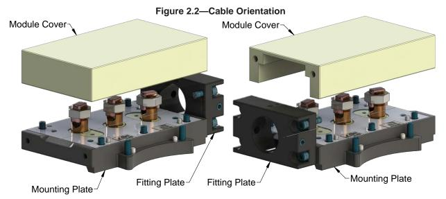
7. Feed the cable(s) through the customer supplied strain relief fitting and prepare the cable ends by stripping the insulation back approximately 3/4" (19 mm) using wire strippers. Be careful not to cut individual strands while stripping the cable insulation.
