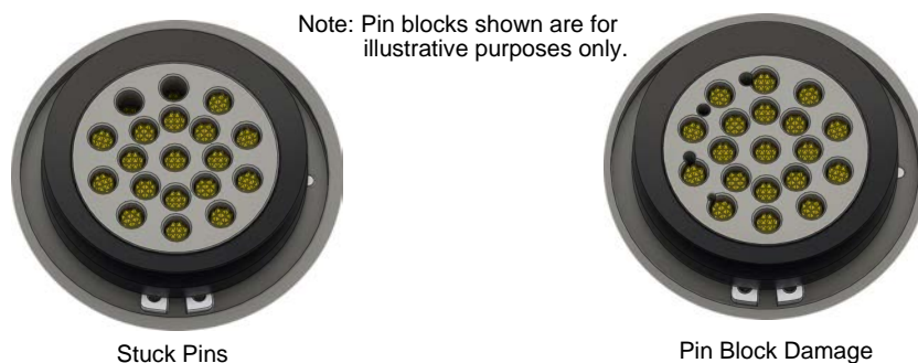
Figure 4.3—Stuck Pin and Pin Block Damage
