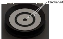
5. If debris or blackened center pin and shielding ring are present, use a vacuum to remove the debris, and clean using a nylon brush (ATI Part Number 3690-0000064-60).
