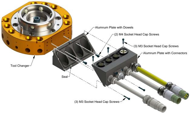
Figure 2.7—SE Module Installation (SE32 Module Shown)
