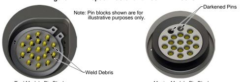
Tool Module Pin Block
