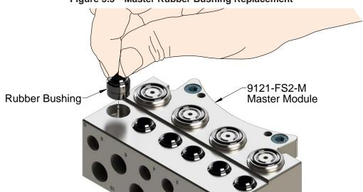
Figure 5.5—Master Rubber Bushing Replacement
