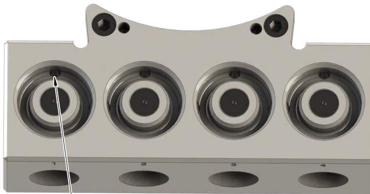
Figure 4.1—Inspect and Clean Drain Holes in Tool Module
