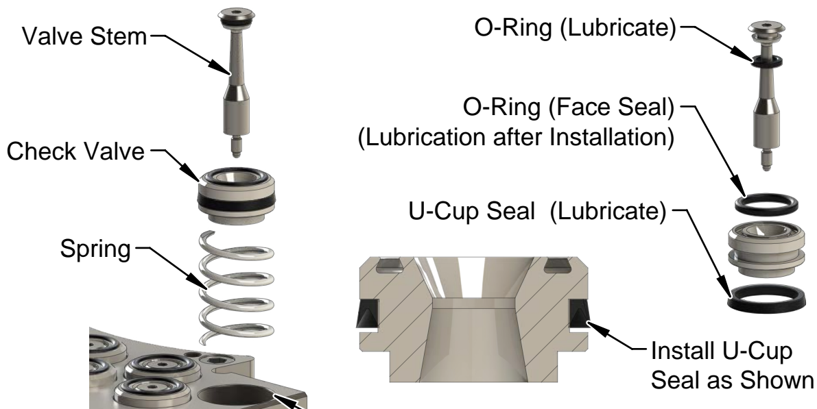
Figure 5.2—Master Self-Sealing Valve Installation
