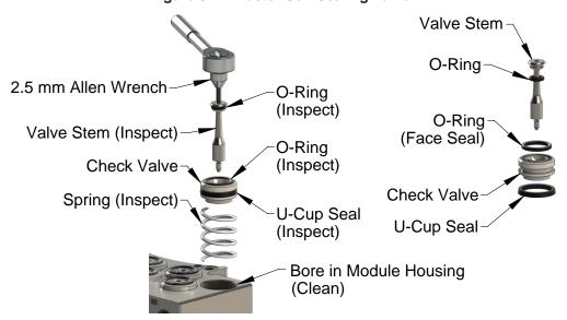
11. Lubricate the bore in the module housing with Magnalube G (Teflon/Petroleum based grease).
