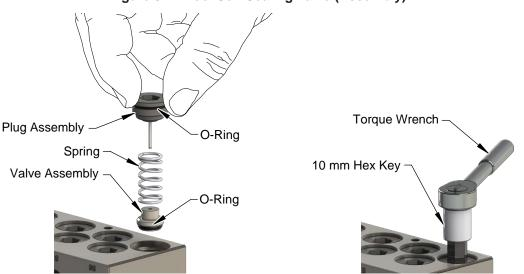
Figure 5.4—Tool Self-Sealing Valve (Assembly)
