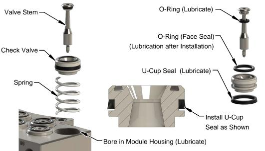
Figure 5.2—Master Self-Sealing Valve Installation
