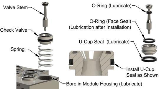
Figure 5.2—Master Self-Sealing Valve Installation
