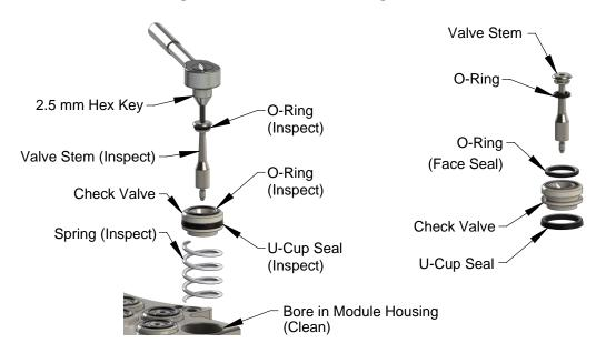
11. Lubricate the bore in the module housing with Magnalube G (Teflon/Petroleum based grease).
