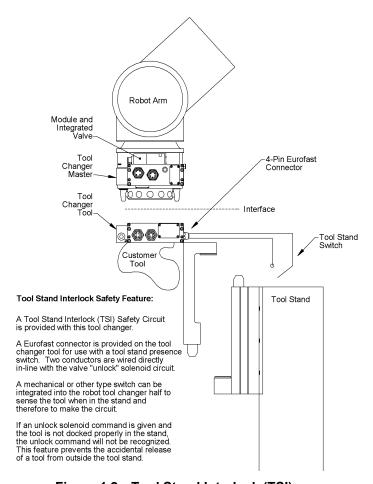
Figure 1.2—Tool Stand Interlock (TSI)
