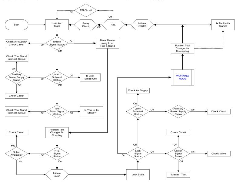
Figure 3.1—Logical Operation and Diagnostics (Shown with Double Solenoid Valve)
