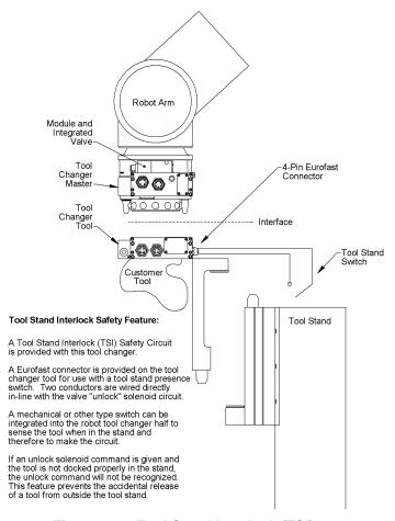
Figure 1.2—Tool Stand Interlock (TSI)
