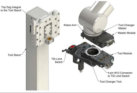
Figure 2.1—Tool Stand Interlock (TSI)
