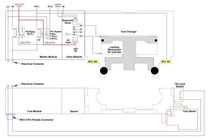
The second set of contacts on the RTL bypass relay is used to provide the RTLV diagnostic signal (when the RTL bypass relay is open, the RTLV signal should be off). The RTLV signal can indicate if the RTL bypass relay is operating properly.
